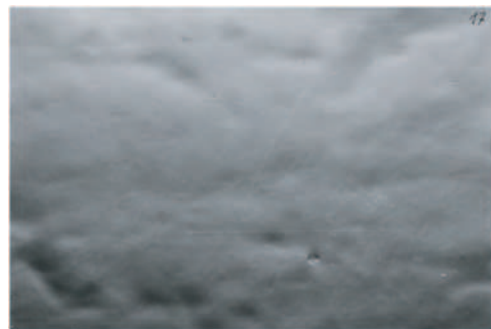
Microscopic view of mechanically polished and electro polished Ra 0,25\text{ }\mu\text{m} / 10\text{ }\mu\text{-inch}
